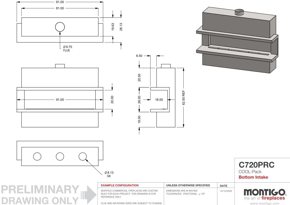
FLUE AND AIR INTAKE SIZES ARE SUBJECT TO CHANGE DEPENDING ON VENT RUN.
